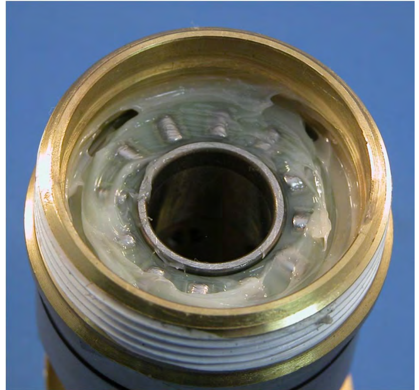
Install thrust section. Add small amount of grease. Add thrust washer. Install onto auger.
